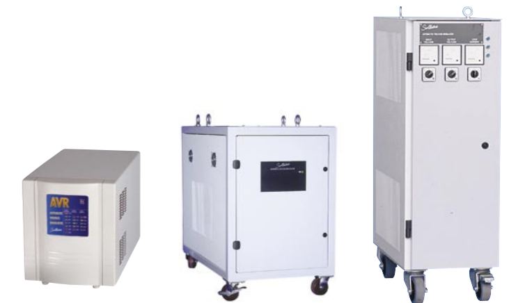
The Sollatek single and three phase AVR range protects against high and low voltage, spikes and surges and has an input range of -30% to +22% as standard.
